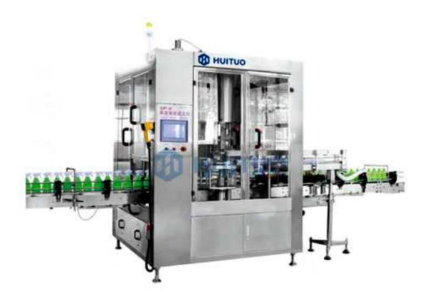
This capping machine has one manipulator, dispatches caps in high speed with no reverse caps which can be suitable for various types of bottles.
