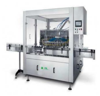
The bottle washing machine is mainly used for washing plastic bottles and glass bottles. It mainly consists of such procedures as elastic mechanical hand bottle grabbing, turning, bottle rinsing, bottle controlling, resetting, bottle discharging, etc. It is equipped with high pressure pump. It adopts continuous tracking washing, achieving fully automatic production.
