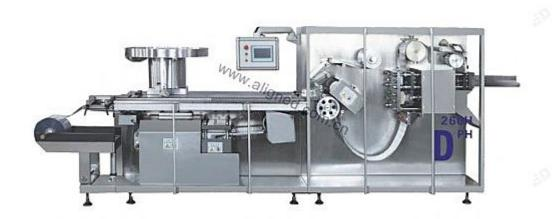
Automatic High Speed Blister Packing Machine DPH-260 combined the stamping and heat sealing roller. The technology is suitable for packaging of sugar-coated tablets, capsules and other drugs. It can also be used for packing items of hardware, electronics, medical devices and food which have a similar shape with the above drugs.
