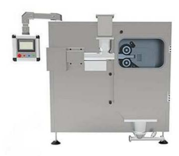
Pharmaceutical Dry Granulator Machine is to mix the dry powder materials by the ingredients, and add them to the upper hopper by a special feeding device (pneumatic or motorized), and send them to the pressure chamber through the screw conveyor. The two high pressure pressing wheels press the material into high density slices. The density slices are granulated to the demanded size by a two-stage granulation system.
