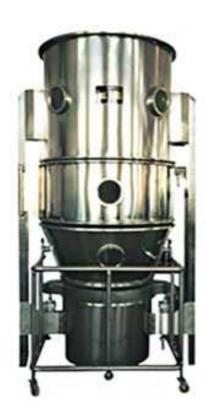
The powder granule in vessel (fluid bed) appears in the state of fluidization. It is preheated and mixed with clean and heated air. At the same time the solution of adhesive is sprayed into the container. It makes the particles become granulating that contains adhesive. Being of unceasing dry through hot air, the moisture in the granulating is evaporated. The process is carried out continuously. Finally it forms ideal, uniform and porous granules.
