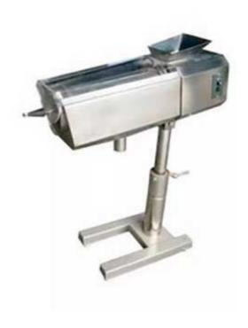
This machine is suitable for dedusting all type of tablets. It is adapted to all types of tablet machine. With the attachment of deduster and compressed air the dust could be got rid of doing the vibration at the filter.
