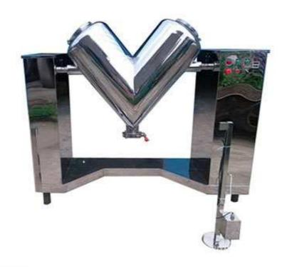
This V shape Mixer Machine is mainly used for mixing powder or granular materials in food, chemical, pharmaceutical and other industries. Unique v shape geometric structure, can achieve efficient uniform mixing. There is no dead corner and no residual material in the mixing process. This Mixing Machine is equipped with a unique stirring paddle, which can mix the raw materials which are caked or contain certain moisture.
