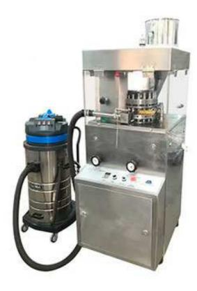
This machine is designed for pressing round tablets or special shapes from various kinds of granular materials. It is primary machine to fit batch production of tablets. The turret carries 19 sets or 17sets of punches and dies, so 19/17 tablets will be pressed for each revolution of the turret. During operation, the speed of the turret rotation, the depth of the filling material and the thickness of the tablets can be adjusted.
