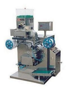
The DSL160 Strip Packing Machine is designed to pack capsules, tablets or similar products.
