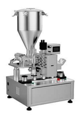
This machine adopts with internal heating method to seal the tube tail, more safer and stabler. Working process requires human intervention and consists of manual color-mark finding, filling, heating, sealing, manufacturing date printing, cutting and tube discharging. It often applies to the cosmetics industry, like face cleansers, hair conditioners, hair dyes, toothpastes, which is suitable for various packaging materials such as hoses, composite tubes, and various sizes of customization.
