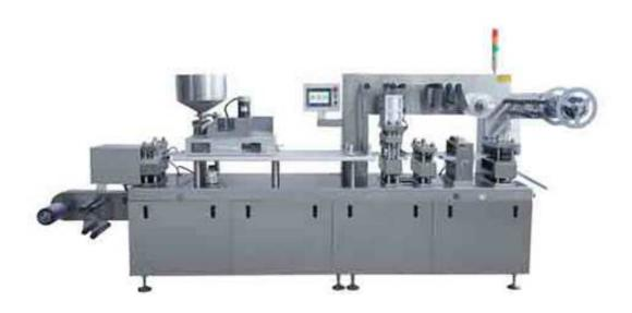
The machine is suitable for capsule, tablet, big honey pill, candy, liquid, paste, syringe as well as irregular shape Al-plastic, paper-plastic composite and Al-Al sealing packing in pharmacy, healthcare, food, cosmetics, medical equipment industry etc, fully comply with "GMP".
