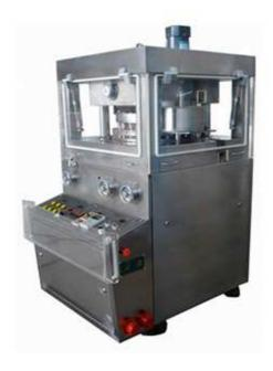
This machine is used to press the granular raw material into the round tablets or various geometric shaped tablets, it is especially caters for small scale production. When pressing the tablets, the rotary disc speed and filling depth of material can be adjustable.
