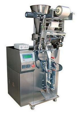
It is used for packing loose, non sticky, granular materials such as instant drink, pellet, monosodium glutamate, sugar, dried soup stuff and oatmeal and like in pharmacy, food and chemical industry.
