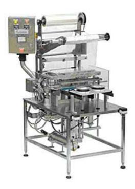
**Performance:** Semi Automatic PAO Line of machines performs membrane cutting and sealing from the roll.
