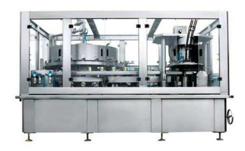
This machine is suit for fill and seam of beer and other carbonated soft drinks, like cola, soda, energy drinks and so on. It adopts isobaric pressure filling principle. The main electric elements adopt "Siemens" PLC, "Delta" frequency converter and "Omron" proximity sensor, "Siemens" analog output.
