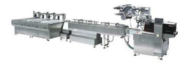
This horizontal packing machine for confectionery products DXD-660/560 is suitable for packing products like chocolate, products coated with chocolate, biscuits, wafer, bread, cakes, and others.
