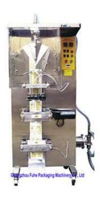
The equipment is widely used in milk, bean milk, various drink, soy sauce, vinegar and wine and so on various film packaging of liquid, ultraviolet radiation sterilization can automatic bag molding, filling, date printing, sealing, cutting one-time finish. The machine adopts stainless steel structure, international health standard. PLC control, photoelectric tracking, perfect design. The stable performance, easy operation, low fault rate. Get the praise of customers at home and abroad.
