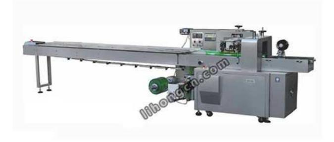
This flow wrapping machine is designed to unitize product packs as well as to individually package piece products in three seal bags ("Flow Pack"). This machine is suitable for irregular shape products as well as normal product.
