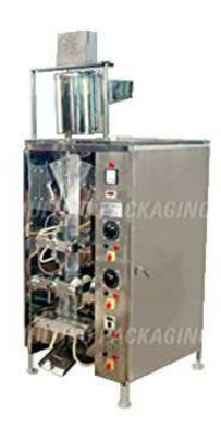
The MK-302 is a vertical form, fill and seal packaging machine designed to package various free flowing liquid products. This Vertical packaging VFFS machine uses LDPE (Poly) film with gravity based filling system to produce center sealed pouches also commonly known as pillow pack or fin seal type pouches / bags.
