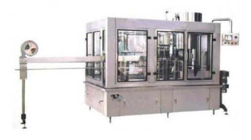
The machine is a full-automatic multiple-function washing, filling and capping unit. It is used in washing. Filling and sealing all kinds of non-air drinks such as fruit juice, oil & vinegar, wine, fruit wine, mineral water and pure water. The line has features of unique design, new style, complete functions, multi-purpose, convenient in operation, beautiful construction, high automatization. It is the best filling equipment in China.
