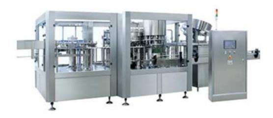
The series equipment is used in hot filling and sealing of green tea, black tea, wulong tea and fruit juice. The machine integrates washing, filling, capping together. The design is scientific and reasonable. Its appearance is beautiful. Its operation and maintenance is convenient. It is good equipment for choosing hot drink filling machine.
