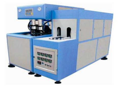
The SH-800 semi-automatic blow molding machine is suitable for blowing PET bottles of various shapes, ranging from 1000 ml to 5000 ml. This blow molding machine is widely used in blowing edible oil bottles, purified water bottles and honey bottles.
