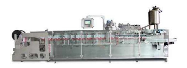
This machine is completely designed with the newest technology, and it has so many different specifications from other machines. It can work with Doypack or 3-4 side sealed pack. It can fill from 200gr to 1500gr. All of the parts made with stainless steel. In optimum conditions it can reach 160 packs per minute. It works with two filling head. For all of the electrical and pneumatic parts world-known brands used. And also this machine has half cut unit.
