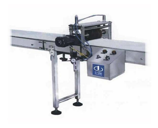
SRJL Leak Detector is designed to check the quality of pre-welding. Inspection is carried out by pressure. This equipment is characterized by simple structure and easy operation. Pressure and speed are adjustable.
