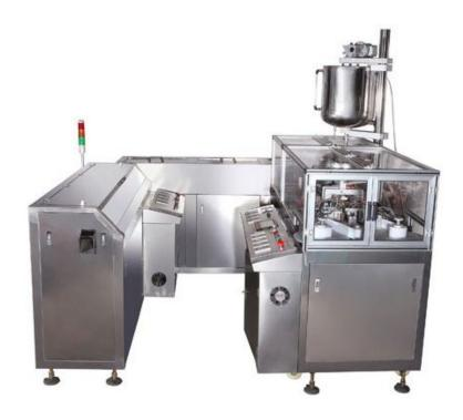
The series of automatic suppository producing line are applied to produce suppository of bullet shape, torpedo shape, duckbill shape and other special shapes filling with materials of fatty glycerides, glycerogelatin and polyethylene glycol.
