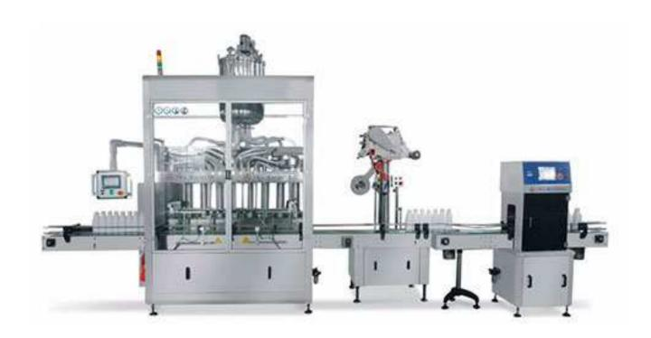
The overflow milk filling machine is filing by feeding pump, the volume is controlled by the level, there is a sensor on the filling nozzle, we can adjust the position of the filling nozzle to control the filling level. Overflow milk filling machine is specially for the high level request, overflow filling machine can fill to the bottle mouth.
