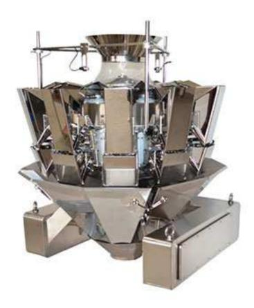
Automatic Granule Paste Multihead Weigher is special design for Paste, extra one hopper in order to increase the speed, for regular products, 10 head weighed may meet the demands of speed 35-60, but the shape of Paste is difficult to run that fast, so we add an extra bucket on it.
