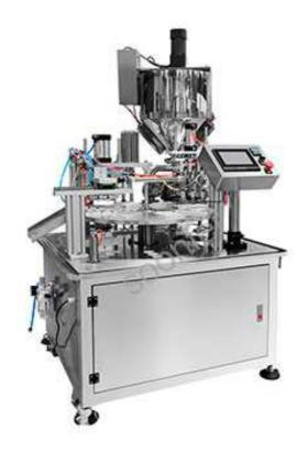
High-speed honey spoon packaging filling machine, filling honey in the shape of a spoon, the spoon can be customized, and can pack 800-1000 pieces per hour.
