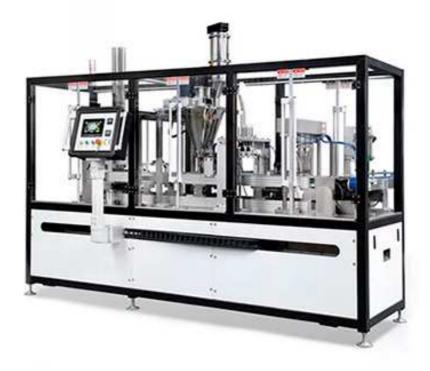
You need better and faster machine to meet your requirements. TRY Our AF-H2 K CUP filling sealing machine. This machine Can produce 2 capsules at a time, with around 80-100 pcs per minute.
