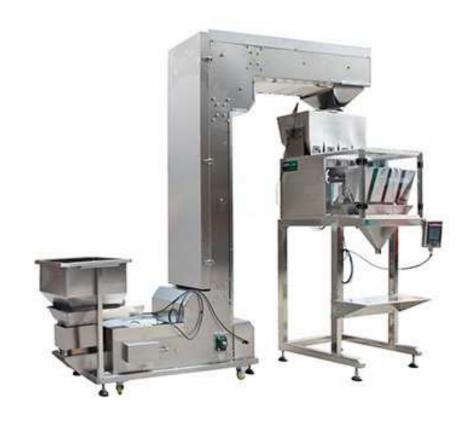
The coffee bean packing machine is design according to national GMP standard. It's able to complete auto-dosing, filling and out-of-tolerance alarm. It's suitable for packing materials such as powder, granule as well as squeezing expanded, absorbent, irregular proportion change material. The range of application: sugar, salt, detergent powder, seed, rice, milk powder, MSG, coffee, sesame seed, and so on.
