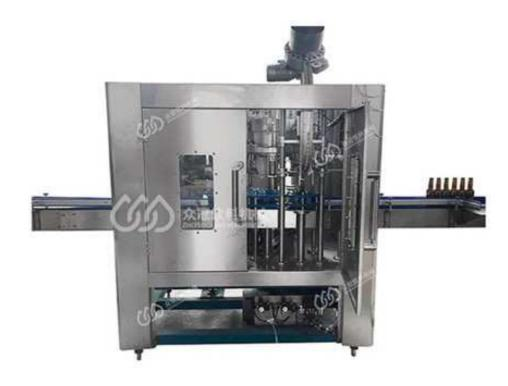
The DXGF carbonated drink filling monoblock is used to fill carbonated drinks into plastic or glass bottles. Washing, filling, sealing can be carried out on the same machine. The design of the machine is scientific and reasonable.
