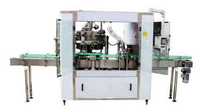
Our newly designed BCGF serious monoblack beer filling machine is designed for aluminum can and metal tin can filling, it can suit for can size between 150ml to 750ml, can customized to maximum of 1000ml. On machine surface is only leaving 3 points of bearing support point which makes drainage so easy and without any dirt stain.
