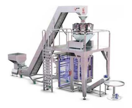
The latest German technology has been used to manufacture this industrial line, such as the compressed air systems, drive and control sensors, and optical sensors, in order to provide good performance, high speed and continuity of work for 24/7. It is equipped for the purpose of packing the (Biscuits- Snacks- Nuts).
