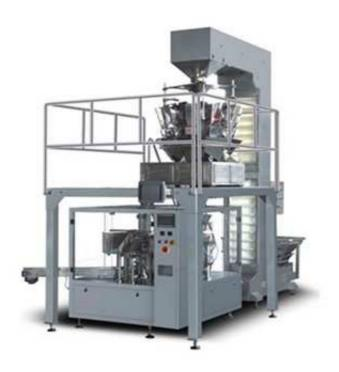
This set of equipment is mainly suitable for automatic counting and packaging of small bags (like medicines, coffee, cereal, cold granules, etc.). After lifting the pouch material into the automatic metering device by the hoist, the computer automatically combines the set quantity, and automatically packs, seals, and outputs the finished product by the bag type packaging machine, and the whole set of equipment is highly automated.
