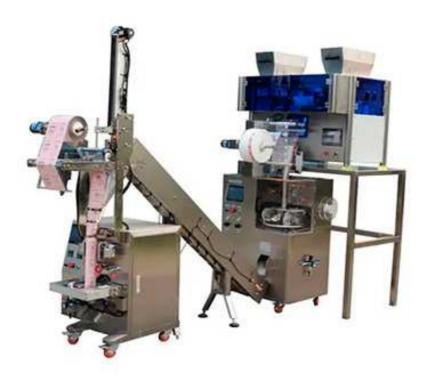
This is our full automatic pyramid tea bag packing machine, it makes triangle / pyramid / rectangular flat shape tea bags automatically, the machine controlled by PLC, and all the parameter setting like tea bag shape changing can be finished on the color touch screen. Outer envelop machine can be added, then you can make pyramid tea bag with outer envelop.
