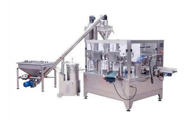
Automatic Rotary Pre-made Bag Packaging Machine is widely used to fill powder, solid products into pre-made bags and seal the bags automatically.
