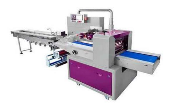
The Down-Film Flow Packing Machine is a large category of packaging equipment, and it is the right hand of many manufacturers. It can be used not only for packaging of unmarked packaging materials, but also for packaging using rolls of materials with logo patterns.
