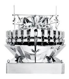
The 32 head multihead weigher is designed to simultaneously weigh two different items with a weight of 10-1000g, making it suitable for various granular, sheet, strip and irregular items. The target weight is freely adjustable to meet customer packaging needs for versatility.
