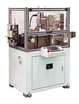
Electronic Embossing Cutter can emboss and cut all kinds of toilet soap and laundry soap, fast and accurate. This machine's control system uses world famous brand PLC, touch screen, servo, encoder, etc. and cam system to make the machine running accurately and reliably.
