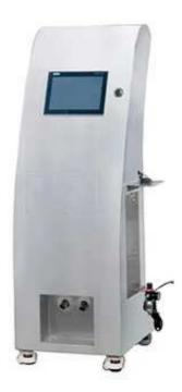
Automatic capsule weighing machine KWS-60 is small equipment which can be connected with the automatic capsule filling machine to check whether the weight of the produced capsules meets the standard.
