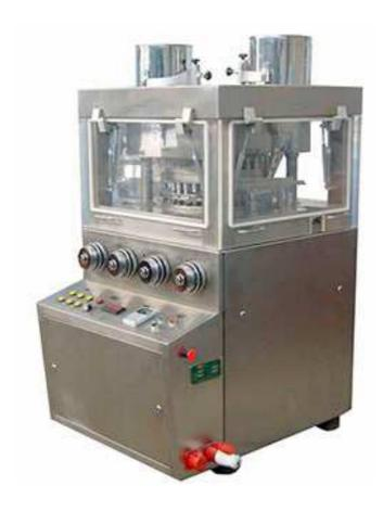
This machine is an automatically-revolving double-pressing piece-pressing machine which could enable the granular active pharmaceutical ingredients (APIs) to be pressed into tablets. It is mainly used to manufacture tablets for the pharmaceutical industry and also suitable industries such as chemical, food and electronic industry. Features
