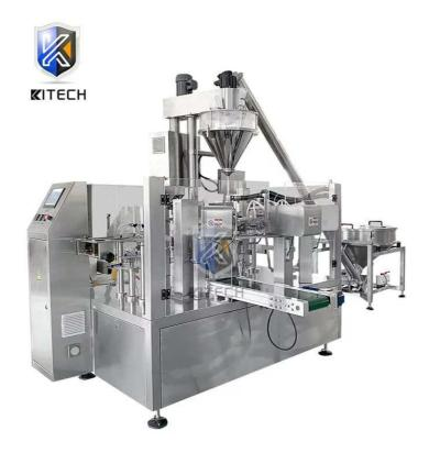
Full automatic premade pouch bagger, featured with rapid reaction, reliability and quick changeover, is ideal for a large variety of bag types and range. Equipped with Auger Filler and Screw Elevator, it is widely applied to packing powder, such as detergent powder, milk powder, flour, spice, coco powder, ground coffee, and so on.
