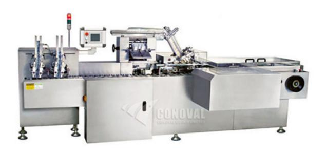
DC180H automatic cartooning machine is intellectualized, continuous fully automatic cartoning machine which can reach speed of 180 cartons/min.
