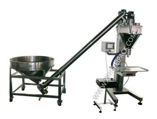
The machine can finish the process of dosing, filing, and alarm of the difference of the weight. The machine is suitable for packing powder material, such as milk powder, feedstuff, rice flour, sugar, coffer, monosodium glutamate, solid beverage, grape sugar, solid medicine, etc.
