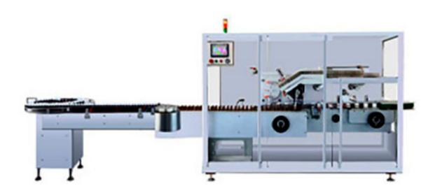
ZH-Series Automatic Cartoning Machine is suitable for automatic filling and packing of products such as granular bags, soft double aluminum, plaster, band aid, facial mask, coffee bag, bottle, aluminum plastic plate and so on.
