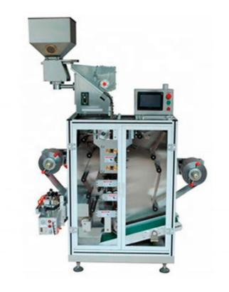
It applies to package the Tablets, capsules and Electronic Components in the pharmaceutical industry. It can make a good sealing and lucifuge well.
