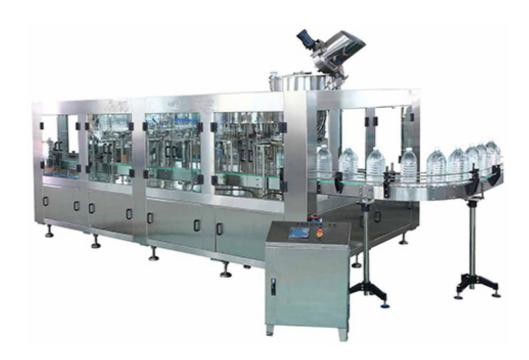
This series of monoblock 3 IN 1 filling machine are applied to the production of 4-8L pure water, mineral water, with optional capacity from 800 to 2 000 BPH. The washing, filling and capping will be finished just by this one machine. It is very convenient to change bottle size by means of advanced bottle conveying technology--bottleneck clamping & bottle suspending technology.
