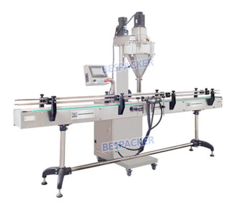
FLG series automatic screw blanking powder filling machine adopts PLC and auger filling mechanism.
