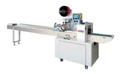
This candy packaging machine ZP-100 is the first invented model, with a stable speed of 220 bags per minute. Horizontal packing using a single film coil with three weldings: two cross-weldings and one longitudinal welding. Automatic candy wrapping machine for high production.
