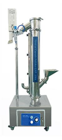
The LFP-150A series capsule polishing machine has the dual functions of capsule polishing and lifting. The entrance of the machine can be connected to any type of capsule filling machine. The outlet can be connected with the capsule sorting device and the metal inspection machine. Realize the continuous production mode of polishing, lifting, sorting and testing. The machine adopts a number of new technologies and human design concepts.
